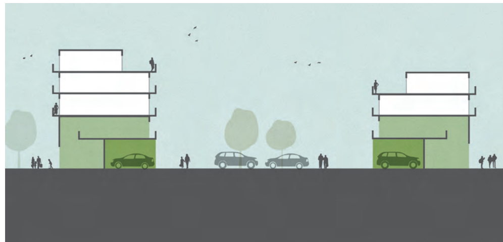
Figure 2.4: Illustration of suitable undercroft parking provision.
